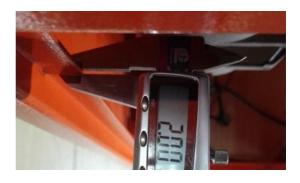
2.0mm cold rolled steel, car paint
