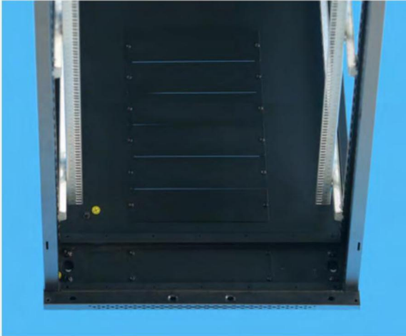
Close the cable entry at bottom
